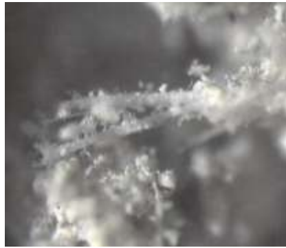
Asbestos fibres in crushed eternit
