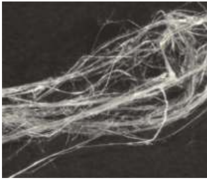
Chrysotile serpentine asbestos
